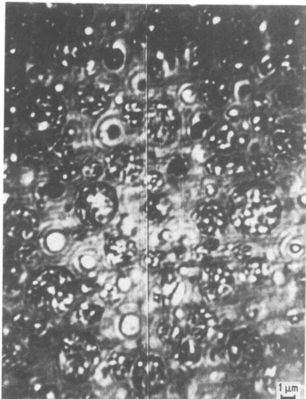
Figure 4 Acoustic micrograph (2 GHz, X-Y mode) of Kerimid 70003 BMI sample showing multi-phase/void structure.
